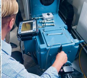
The course is organized for maintenance technicians from ropeway operating companies in collaboration with the companies SPM Instrument Int. GmbH and Spalt Elektromechanik und -maschinenbau GmbH. Participants gain an overview of the early warning signs of equipment failure and of which measured values, such as vibrations and temperature, can be used for diagnostics.
